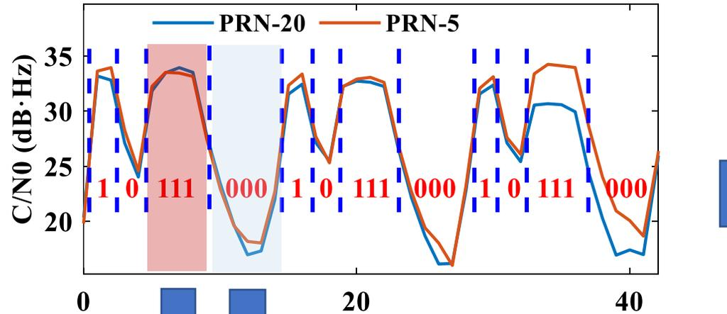
$C/N_0$  measurements of scattered GPS signals
