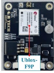
Figure 13: GNSS Module.
